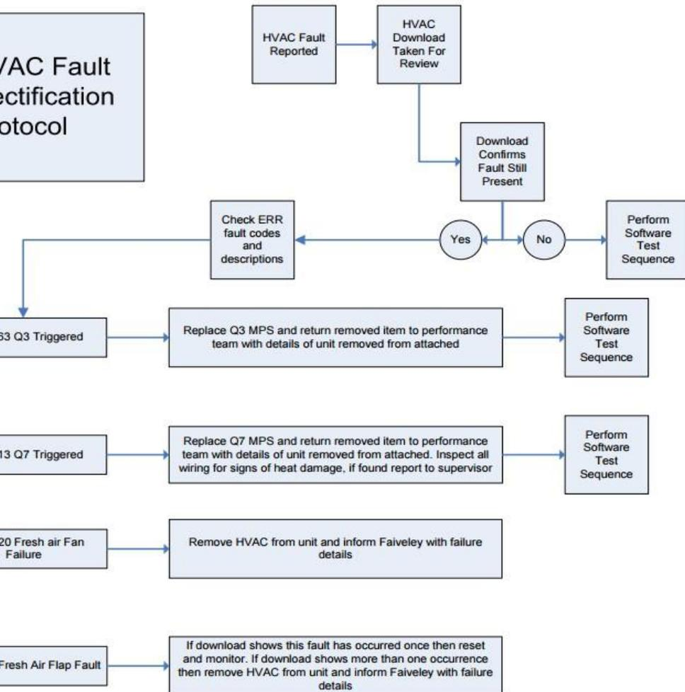
This flow tree is intended to cover the most common faults and actions required for them. Any other faults and fault codes found during fault diagnosis require investigation as per instruction given by Faiveley in accordance with training course.
